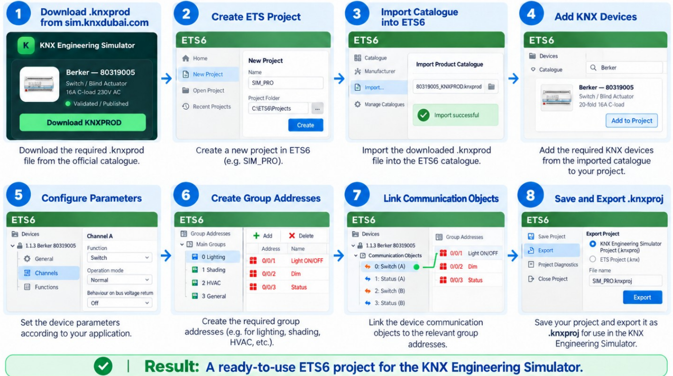
Figure 1 - ETS6 workflow: from catalogue download to .knxproj export.
